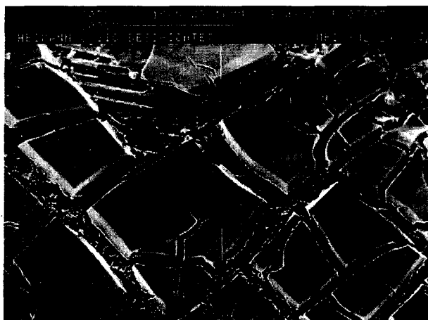
Fig. 4. Ceramic layer on C/C-SiC substrate; prepared by dip-coating with a 67 wt% solution of NCP 200 in toluene and followed by pyrolysis up to 1100^\circ\text{C} ; withdrawal speed = 2.7 \text{ cm min}^{-1} .
