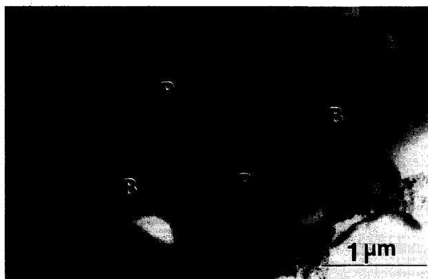
Fig. 13. BF TEM image of Zn-doped BZS pyrochlore ( \text{Bi}_{3/2-x/2}\text{Zn}_{1+x}\text{Sb}_{3/2-x/2}\text{O}_{7-x} , x = 1.2 ) sintered for 4 h at 1035^\circ\text{C} showing large spinel grains (Sp) with pyrochlore (P) and Bi-rich phase (B) with EDS analysis from spinel.
