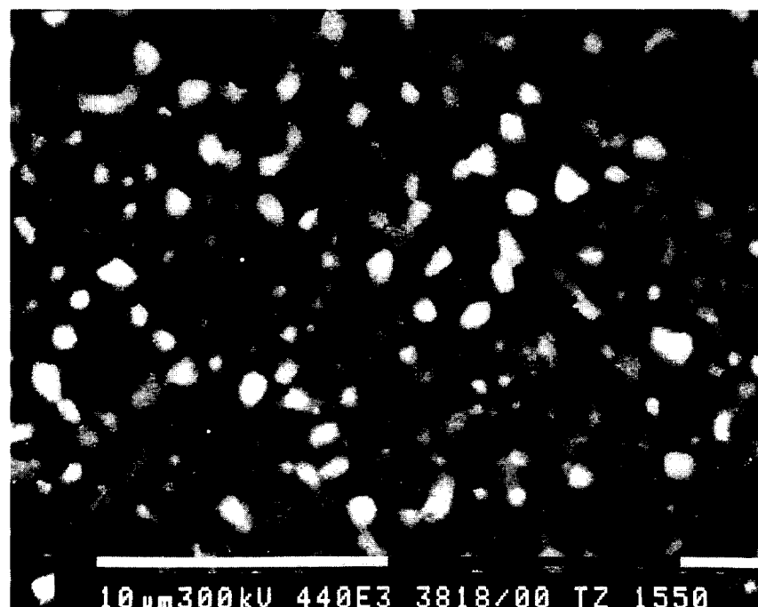
Fig. 8. SEM micrograph of sample TZ sintered at 1550°C for 12 h.
