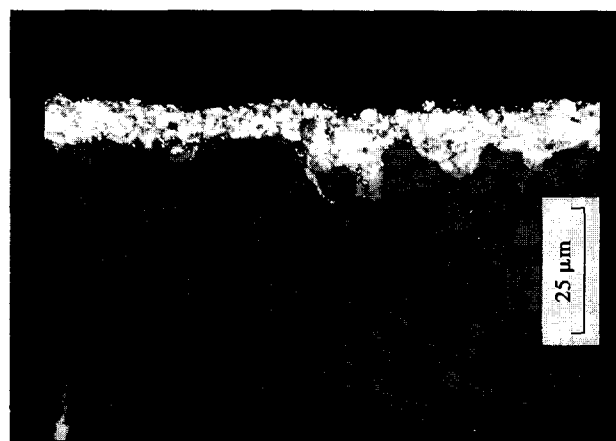
Fig. 6. Cross-section of the coated C/C-SiC specimen, prepared by dip-coating with a 60 wt% solution of NCP 200 in toluene, 45 vol% silicon powder; pyrolysis up to 1100^\circ\text{C} ; withdrawal speed = 2.7 \text{ cm min}^{-1} .
