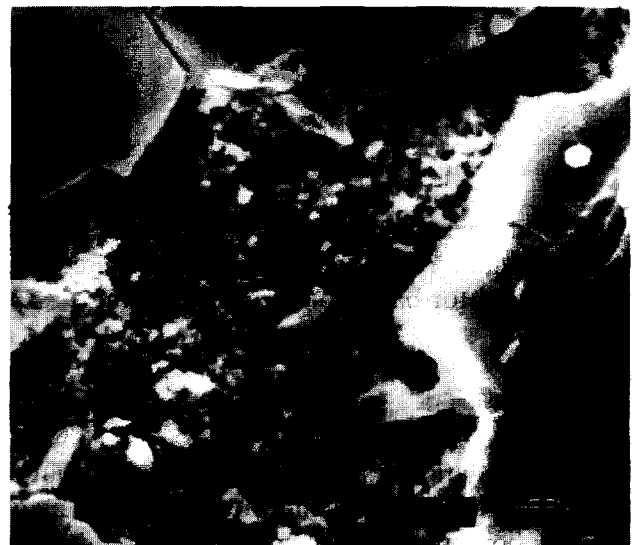
Fig. 5. SEM micrograph of HPSN sample after oxidation tests at 400°C and 30 MPa water pressure.
