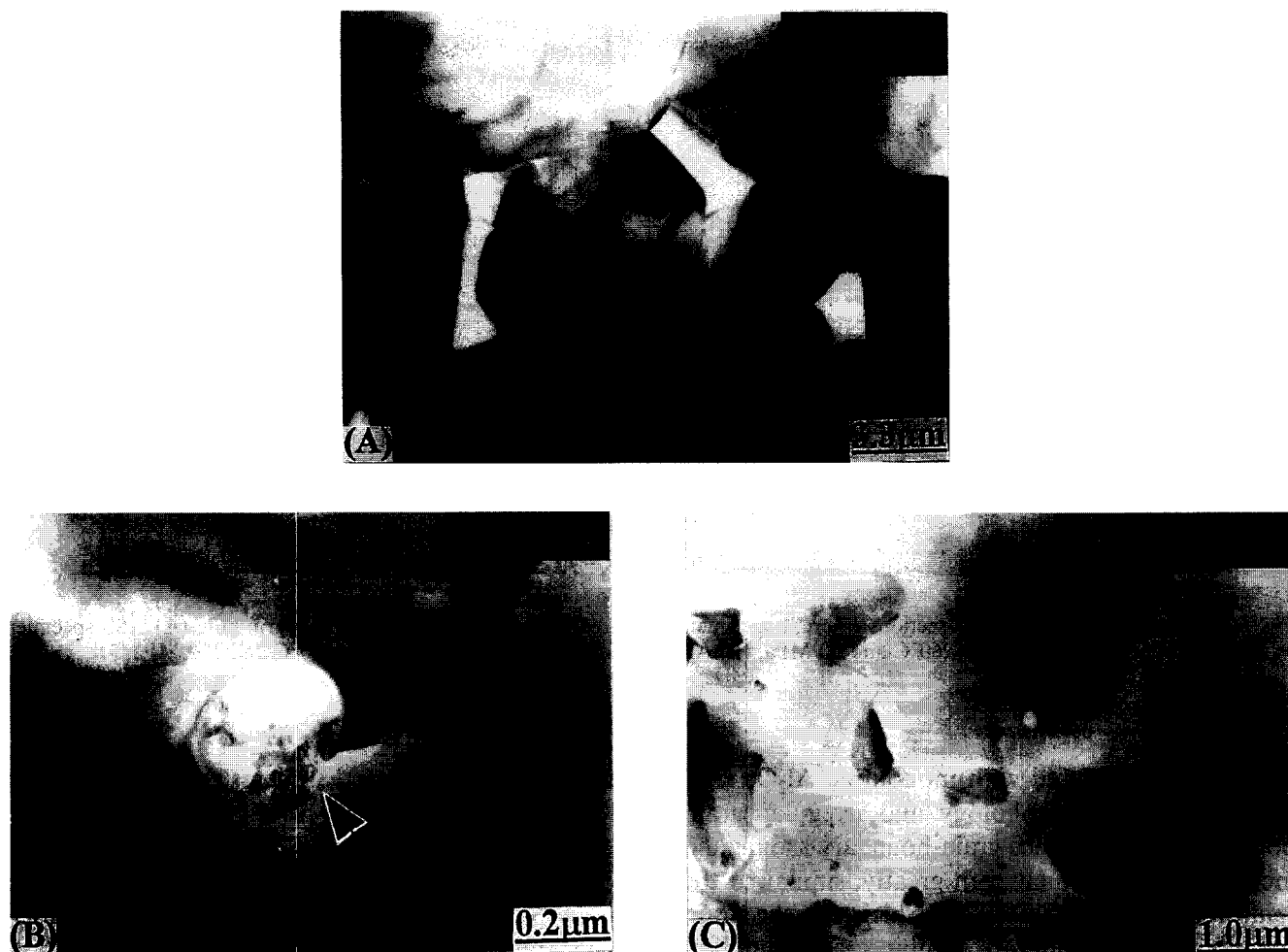
Fig. 5. TEM micrographs of samples taken from the tensile side of crept specimens: (A) monolithic Al 2 O 3 crept for 73 h at T = 1260^{\circ}\text{C} and 50 MPa with creep strain of 2.27%; (B) ASS specimen crept for 71 h at T = 1260^{\circ}\text{C} and 50 MPa with creep strain of 1.23%; (C) ASL specimen crept for 88 h at T = 1260^{\circ}\text{C} and 100 MPa with creep strain of 0.53%.
