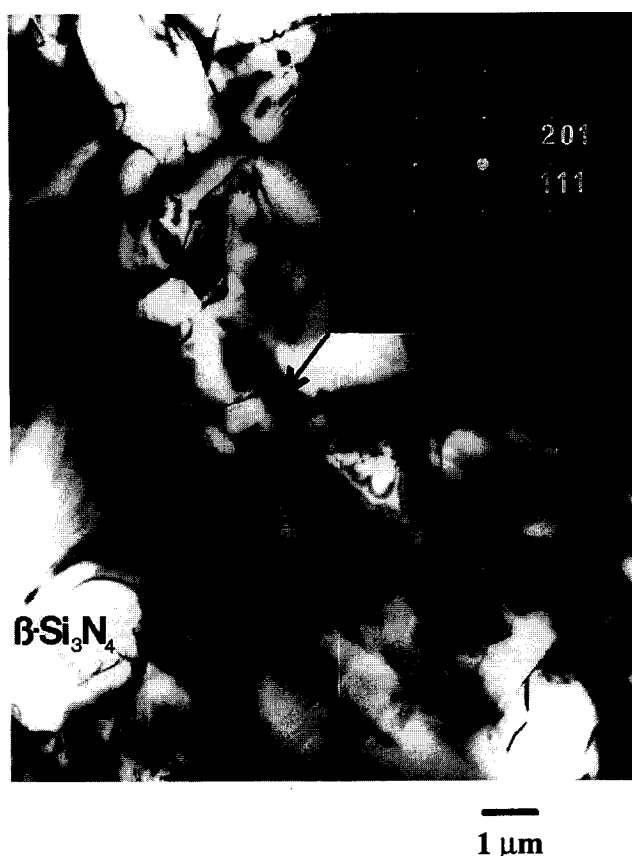
Fig. 4. TEM microstructure of a GPS-fabricated ceramic from run no. 6 (see Table 1), with electron diffraction pattern identifying the melilite intergranular phase.
